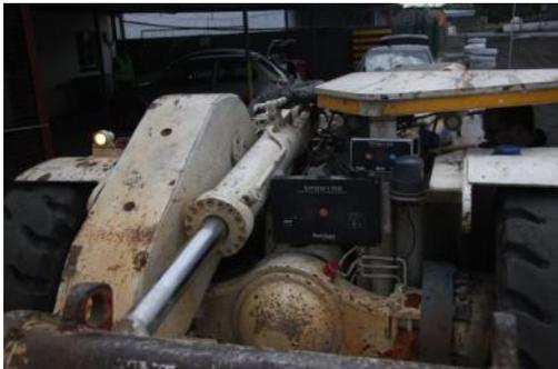
EPOD/RPOD's installed near the scoop. The EPOD signal is not affected by the scoop position.
