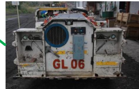
EPOD/RPOD's installed on rear of vehicle in a protected position.
